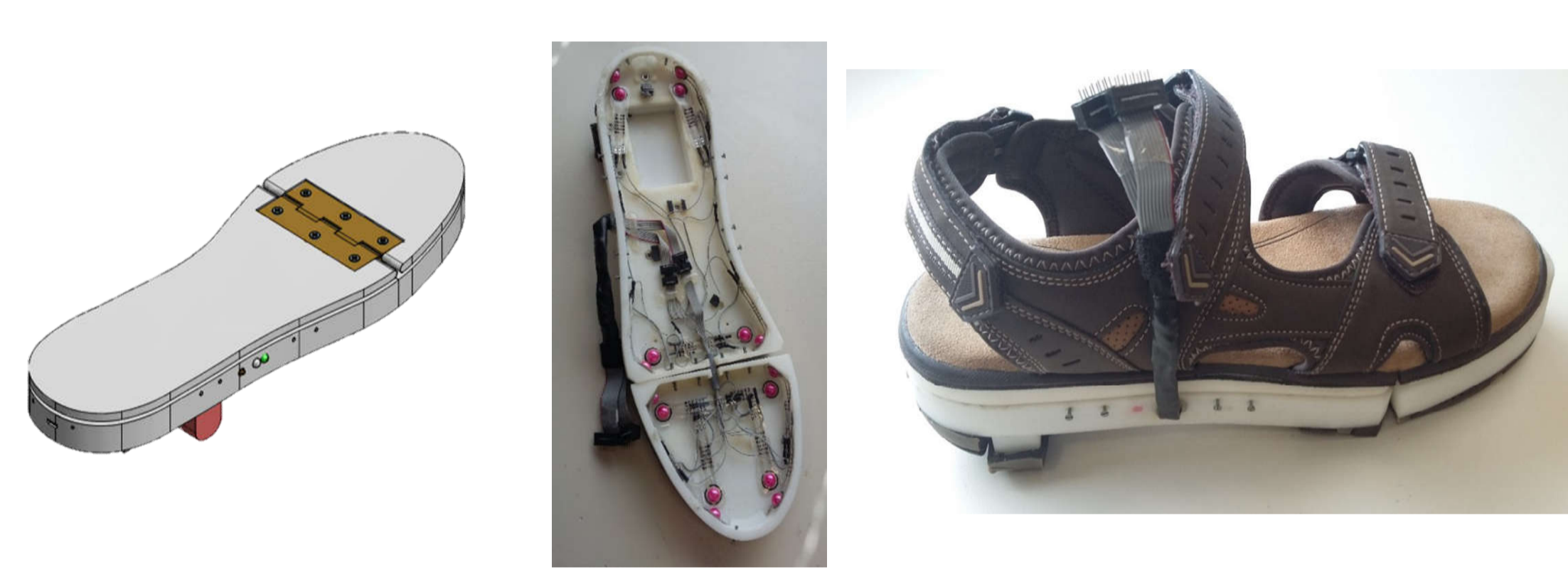
Schematic representation and real instrumented shoe's sole.
